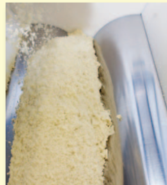
Dough level is automatically maintained in the hopper for consistent dough density in the final sheet.
